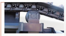
Reinforced hardness of the track guard (3ea for each side).
